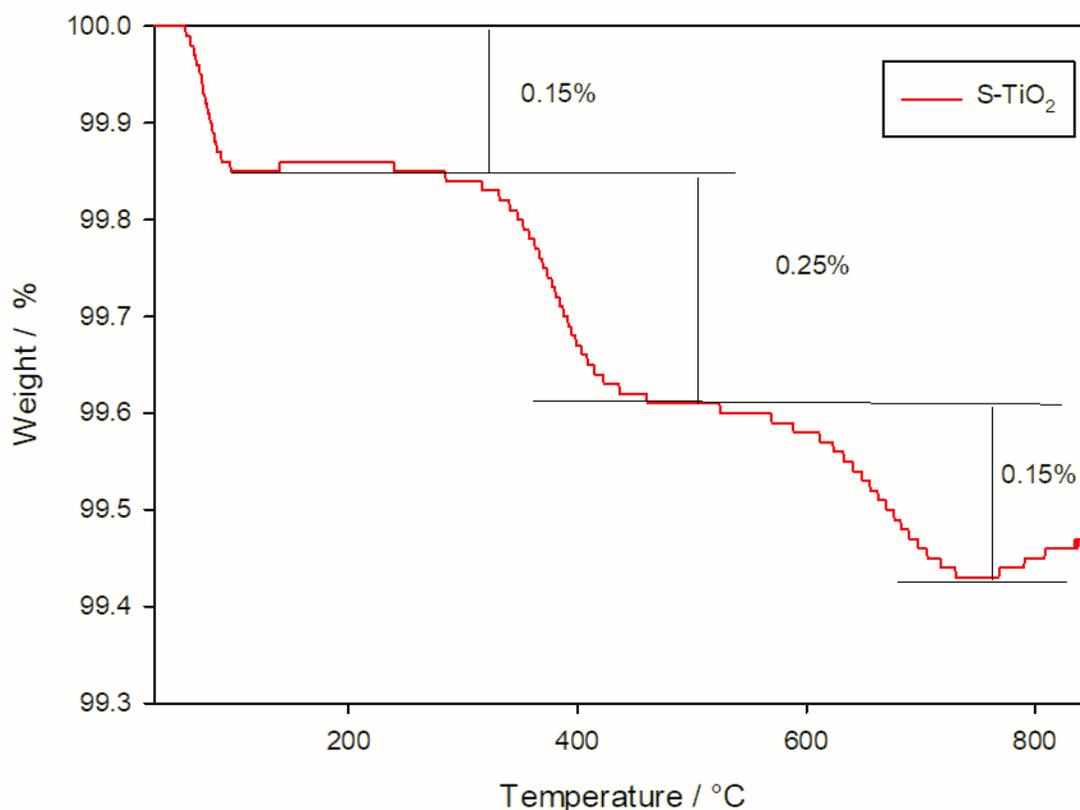
**Fig. 4.** Thermogravimetric behavior of the silanized particles.
