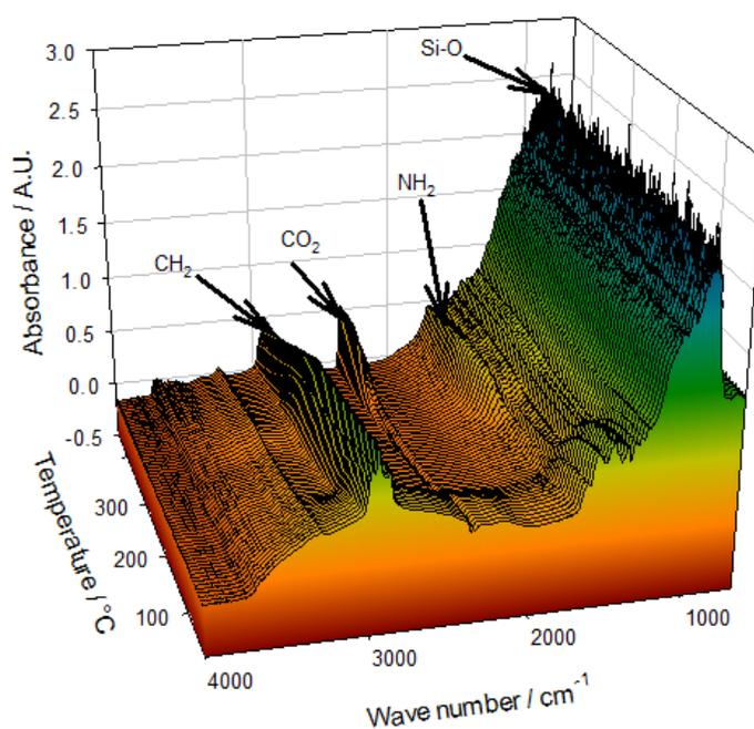
**Fig. 1.** Infrared spectra of silanized titanium dioxide particles.
