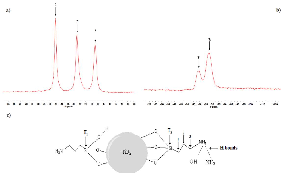
**Fig. 2.** RMN spectra of silanized titanium dioxide particles. a)  $^{13}\text{C}$  and b)  $^{29}\text{Si}$ . C) Proposed scheme for silanized titanium dioxide particles.
