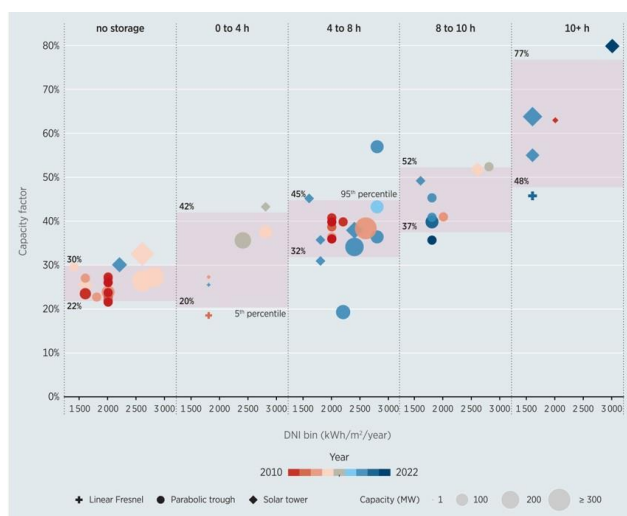
Fig. 2. Capacity factor trends for CSP technologies by direct normal irradiance and storage duration, 2010-2022. From [15].
